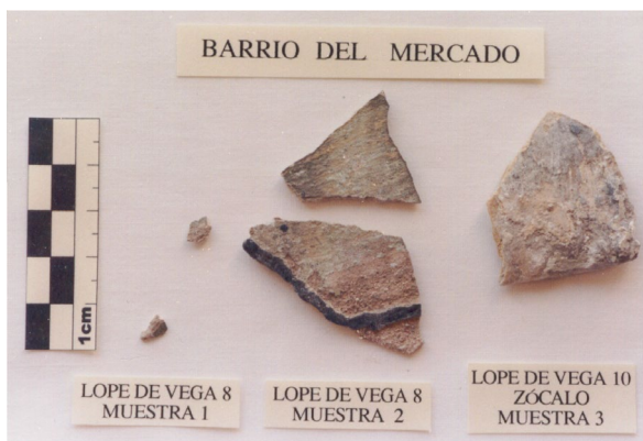
Image n°3: Obtained samples of the plasterings and residual paintings of the facades
