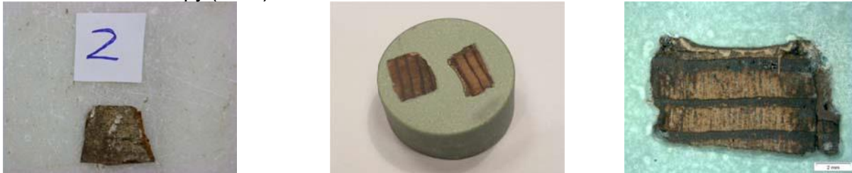
Figure 3: Wood samples and specimen preparation for its microscopy observation.
