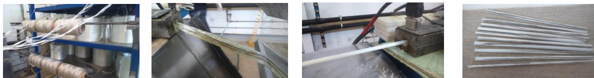
Figure 2. Different phases of pultrusion process obtained by hybrid fibers (flax and glass).
