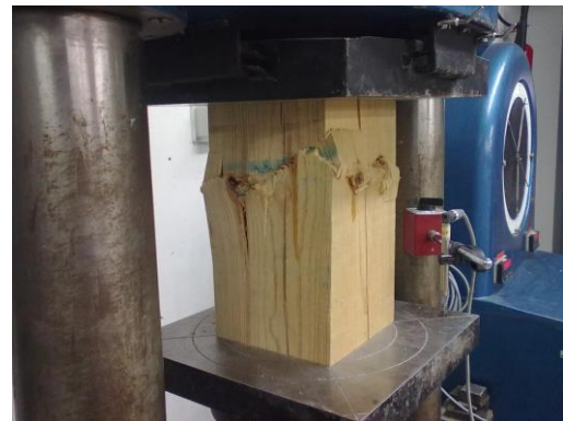
Fig. 1: Compression test of a non-reinforced specimen.
