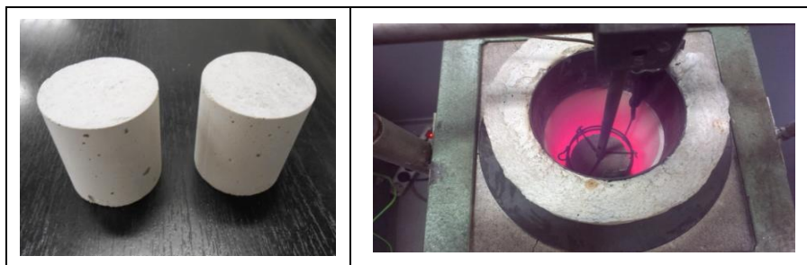
Figure 1. Non-combustibility furnace at work with a sample inside. Detail of a tested sample.
