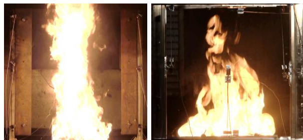
Figure 4 Full-scale experiments of point (left) and frame (right) supported glass façades (fire at the center of glass pane)
