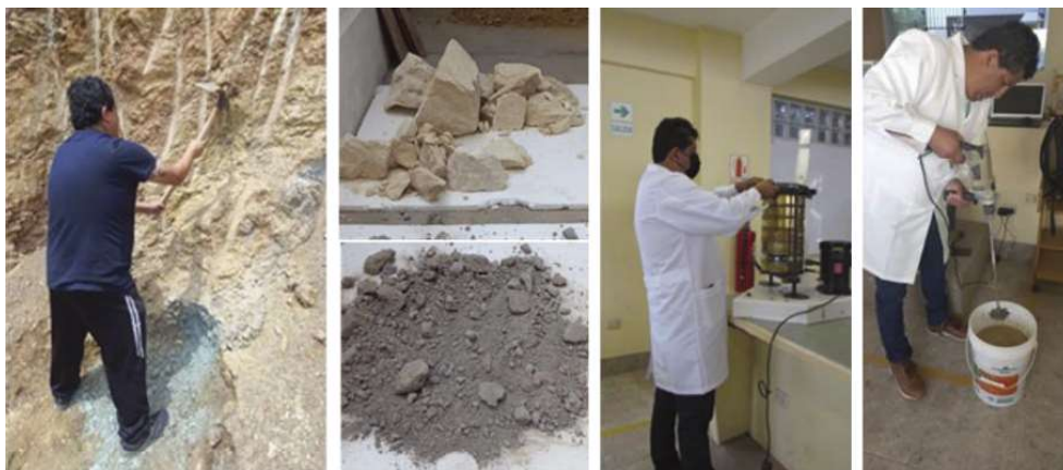
Figure 2: Process of extraction, crushing, sieving and production of inorganic pigments.
